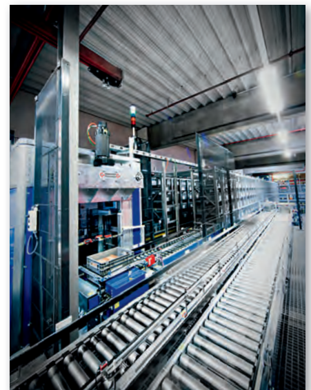
Perfectly networked. Our long conveyor system brings the items included in an order to the correct packing station.
