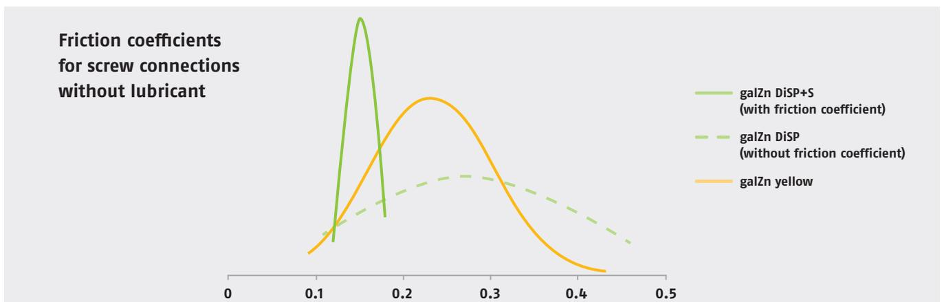
REYHER supports users in the preparation of high quality screw connections with a stock of fasteners ready for despatch with friction coefficient windows set.
