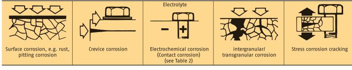
Corrosion is unavoidable, but damage due to corrosion is avoidable, provided the proper planning of suitable corrosion protection measures is in place. The corrosion protection of screw fastenings needs to be at least as corrosion-resistant as the components to be connected.
