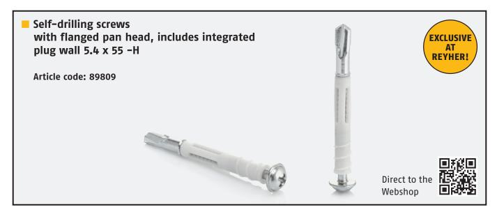
REYHER have a drywall fastening system fastening that is exclusively available in Germany and in many other European countries. This article is a combination of a flanged pan head screw in combinatio with a wall plug. This fastener does not require pre-drilling or additional tools. This means that the screw can be screwed into the drywall in a single step within a few seconds.
